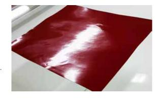
Clear flexible vinyl films can also exhibit mottling, especially when overlaid on a dark graphic. The same measures used to clear
